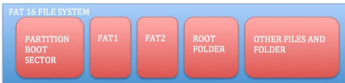
Figure 4.4 FAT16 File System Structure
